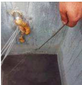
Extracting inner tank temperature sensors
